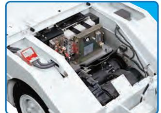
The simple-structured AC system and wide hatch offer easy maintenance.
